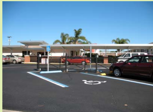
The accessible parking space west of the fence is not connected to the building with a crosswalk
