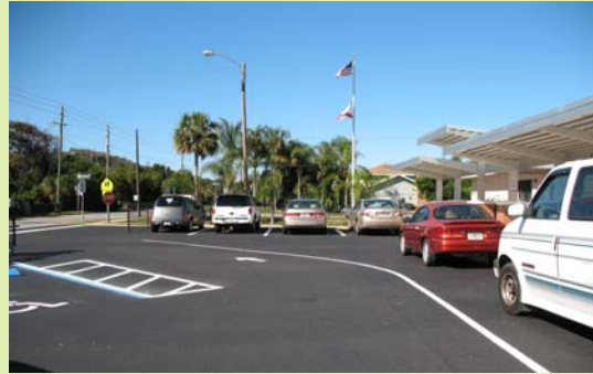
The accessible parking space east of the fence is not connected to the building with a crosswalk
